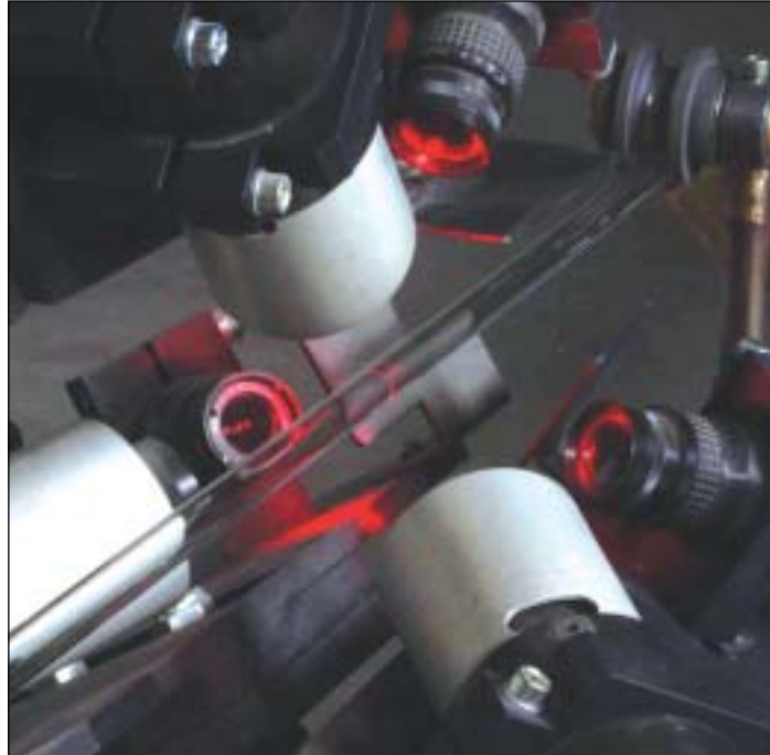
Glass tube inspection
